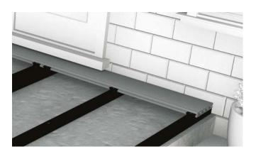
Our Composite Boards are easily fastened to the Joists of a supporting substructure with the help of our Stainless Steel Screws and plastic T-Clip System. Start at the outside of the area to be decked. Place your first Board and fix it to each Joist it crosses using a row of Starter Clips.
