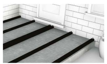
A Starter Clip needs to be fixed to the end of the Composite Joists before laying the first Board. Place these at the end of each Joist where you will start to lay your Boards, leaving a gap of 15mm between the wall and the end of the Joist to allow for expansion.
