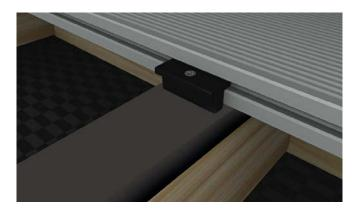
4 Slot T-Clips into the groove along the side of the Board and screw them into the supporting Joists with the screws provided, using one T-Clip for each supporting Joist. We recommend you use our Stainless Steel Wood Screws offering increased wear and less corrosion. T-Clips will leave a 7mm gap between Boards.
