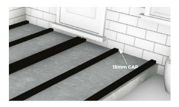
2 A gap of at least 15mm should be left between the ends of Joists and a fixed object such as a wall, and at least 8mm between the ends of Joists at butt joints. These allow for proper drainage and temperature expansion.
