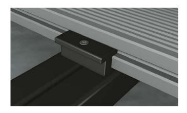
Slot T-Clips into the groove along the side of the Board and screw them into the supporting Joists with the screws provided, using one T-Clip for each supporting Joist. We recommend you use our Stainless Steel Wood Screws offering increased wear and less corrosion. T-Clips will leave a 7mm gap between Boards.
