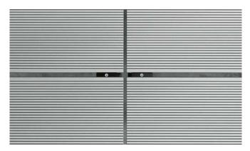
At butt joints - where the ends of two Decking Boards meet, this may mean doubling up on supporting Joists, as you will need to ensure that each Board is held in place with its own T-Clip where they meet.
