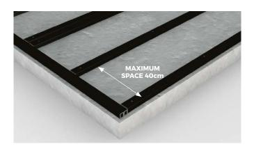
Boards must not be laid directly on the ground but should be fixed to the Joists. The maximum recommended space between Joist rows depends on the angle at which you intend to lay your Boards in relation to the Joists, but should never exceed 40cm, please see diagram Composite Joists should be screwed into the concrete base.
