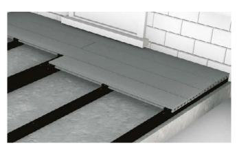
Fit your next Board by sliding it onto the T-Clips used to secure the first Board and fitting another set of T-Clips to secure the opposite side of the Board, using one T-Clip for each supporting Joist. Follow a similar process to fix subsequent Boards. The ends of Boards must be fully supported. No overhang or cantilever is advised.
